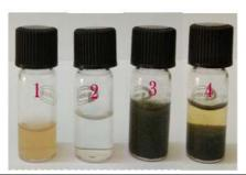
Fig. 3. The images of reactants and reaction mixture during the formation of AgNPs
