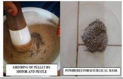
Fig-5: Grinding of surgical mask pellet to powder form
